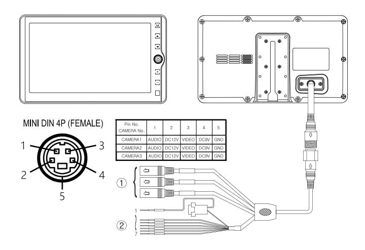
The A/V controller is designed to allow the installation of optional additional monitor.
